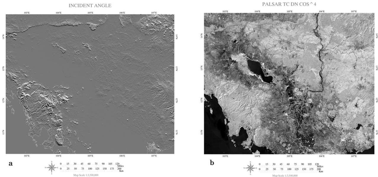
**Figure 2.** Incident angle based on slope and aspect image of SRTM-DEM data (a) and PALSAR terrain corrected image (b).
