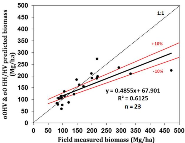
**Figure 6. Relationship between PALSAR predicted biomass plotted against field measured biomass.**
