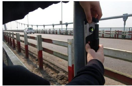
Fig. 8. Conventional measurement using digital spirit level for comparison with TLS results.
