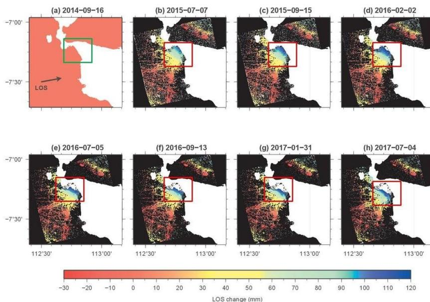
**Figure 5.** Surface Deformation Time Series Result
